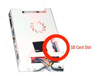
The SD Card on this system can be found on the main Pandora's Box unit as shown above (inside the console cabinet).
